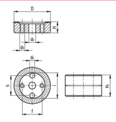
$$\begin{array}{lll} D & = 40 \\ d & = M8 \\ d1 & = 6.3 \\ d4 & H11 & = 6 \\ f & = 23 \\ f1 & = 23 \\ H & +/-0.9 & = 11.5 \\ H1 & = 23 \end{array}$$
